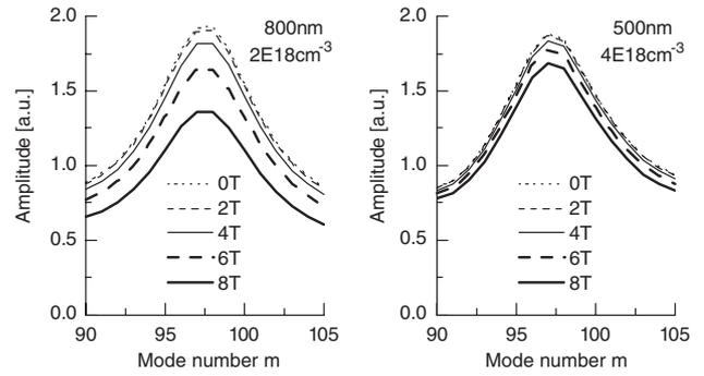
**Figure 2.** Maximum amplitude versus resonator mode number simulation results for two different  $n^+$  layers.
