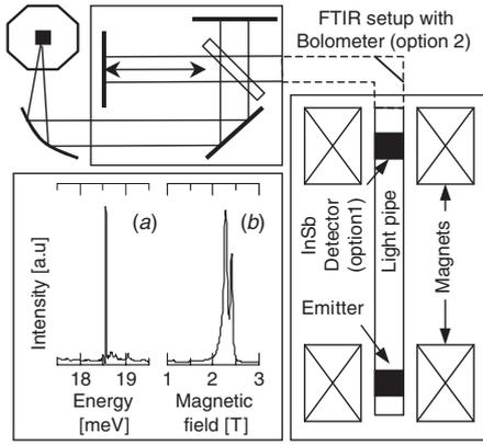
**Figure 1.** Set-up for high resolution spectral measurements: cryostat with superconducting magnets, high resolution (0.0155 meV) Fourier spectrometer and Si-bolometer. (a) High-resolution spectrum of the laser without applied magnetic field at the emitter sample. (b) Response of the InSb detector versus applied detector magnetic field when illuminated by the THz laser (one line corresponds to the free electron cyclotron resonance, the other one to the impurity bound resonance).
