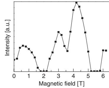
**Figure 3.** Maximal laser emission intensity versus magnetic field. Laser emission intensity was recorded for every given magnetic field flux density value by adjusting pulse generator settings to obtain the maximum intensity. Clear emission intensity maxima are observed for  $N = 2.5$  (4.2 T) and  $N = 3.5$  (3 T).
