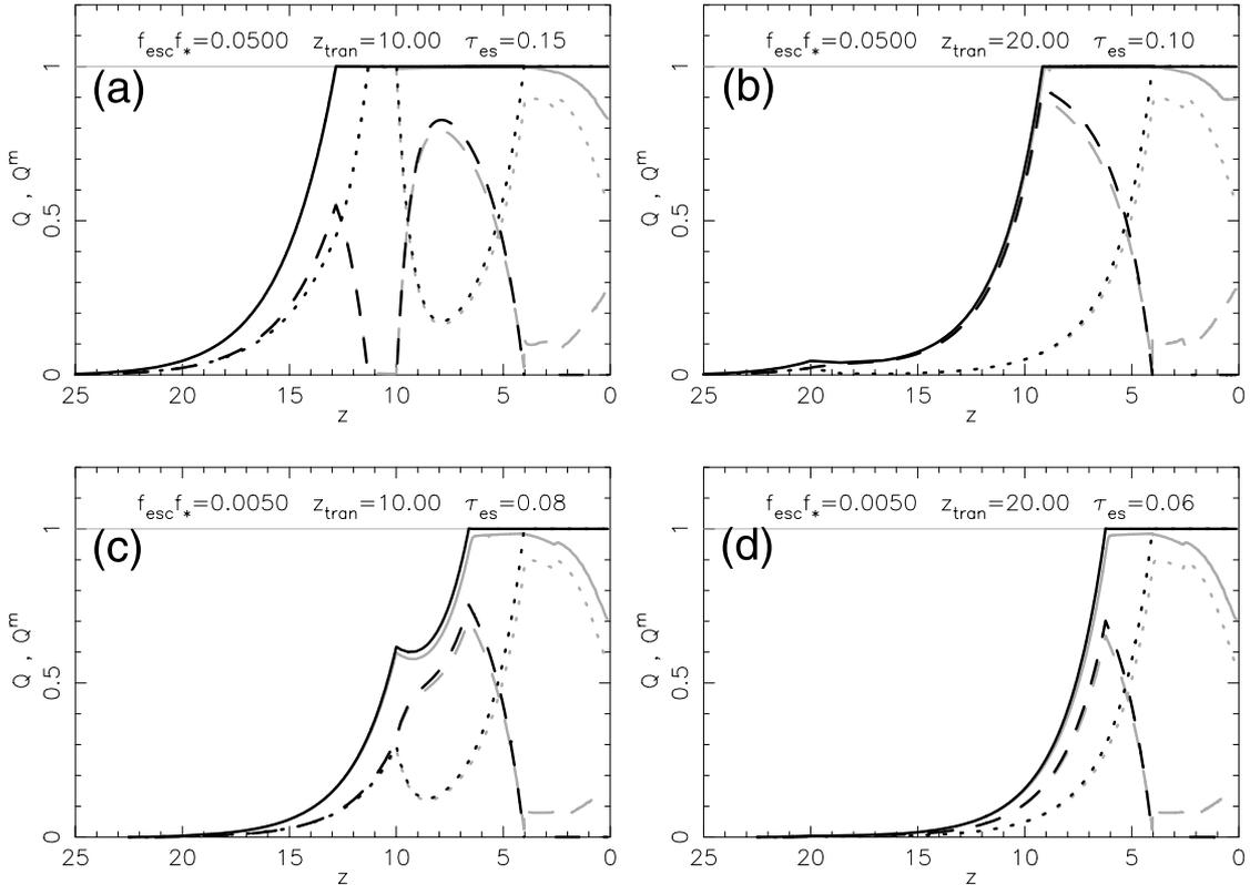
FIG. 3.—Sample reionization histories assuming case B star formation. Dark lines represent the evolution of the volume filling factors  $Q_{\text{H}^+}$ ,  $Q_{\text{He}^+}$ , and  $Q_{\text{He}^{++}}$ , while the light lines show the evolution of the fractions of ionized mass in the universe  $Q_{\text{H}^+}^m$ ,  $Q_{\text{He}^+}^m$ , and  $Q_{\text{He}^{++}}^m$ . The solid, dashed, and dotted lines refer to  $\text{H}^+$ ,  $\text{He}^+$ , and  $\text{He}^{++}$ , respectively.
