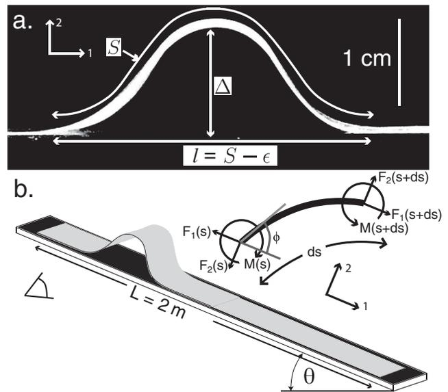
FIG. 1. (a) A ruck in a thin latex rug on a flat substrate, of height  $\Delta$ , length measured along the arc  $S$  and horizontal extent  $S - \epsilon$ . Here  $\epsilon$  is analogous to the Burgers vector. (b) A schematic shows the ruck on a plane at an angle of inclination  $\theta$ . The upper right hand corner shows the local stress and moment resultants for a segment of length  $ds$ , where  $\phi$  is the angle between the local ruck tangent and the plane.
