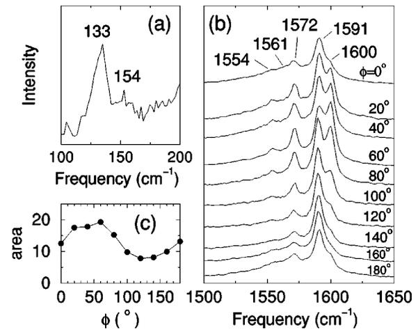
FIG. 3. (a) Raman spectrum of the RBMs for one light spot on the sample. (b) The  $\phi$  dependence of the G-band Raman spectra in the same spot as (a), with the G-band mode frequencies displayed ( $\text{cm}^{-1}$ ). (c) The  $\phi$  dependence of the G-band integrated intensities (arb. units) in (b).
