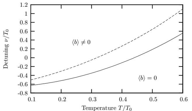
FIG. 1: Phase boundary with detuning  $\nu$  and temperature  $T$ , for fixed particle numbers  $N_f/N_b = 1.11$ . The dashed line has vanishing coupling and has been found with a purely classical analysis. The solid line has dimensionless coupling  $\gamma^2/T_0 = 2.5 \times 10^{-4}$ , and has been determined using the mean-field theory of Section IV. For both, the condensed phase is on the left-hand side (for lower  $T$ ) and labeled by  $\langle b \rangle \neq 0$ .
