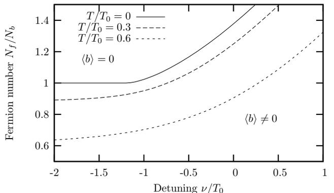
FIG. 2: Phase boundary with fermion number  $N_f$  and detuning  $\nu$ , for three different temperatures. The coupling is  $\gamma^2/T_0 = 2.5 \times 10^{-4}$  and the masses are equal,  $m^f = m^b$ . The two phases are labeled as in Fig. 1, with the condensed phase favored for higher detuning, lower fermion number and lower temperature.
