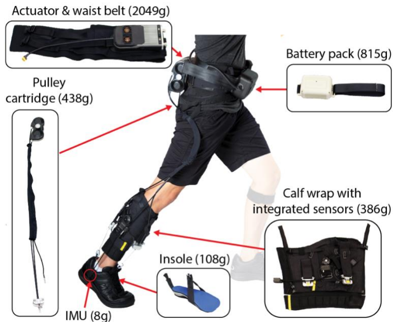
Figure 6.2. Exosuit hardware components and their masses
