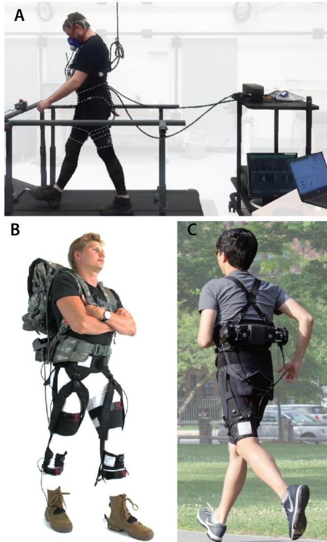
Figure 1.2. Soft exosuit to reduce metabolic cost of transport in healthy walking and running. (a) Tethered exosuit to assist with hip extension using an offboard actuation unit for treadmill-based study (b) Portable exosuit for multi-joint assistance (hip extension and flexion, and ankle plantarflexion) in healthy walking (c) Portable exosuit for hip extension assistance in healthy walking and running.
