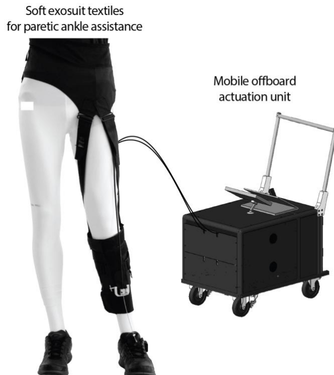
Figure 2.1. Soft exosuit prototype for paretic ankle assistance with a mobile off-board actuation unit. The exosuit uses garment-like functional textile anchors worn around the waist and calf and Bowden cable-based mechanical power transmissions to generate assistive joint torques to the paretic ankle. One end of the Bowden cable is connected to the mobile off-board actuation unit, and the other end is connected to the exosuit textiles. The off-board actuation unit contracts the Bowden cables by changing the motor position, resulting in torque generated at the ankle.
