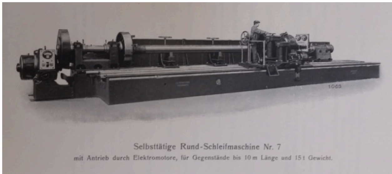
Figure 17: Operative with an automatic grinding machine in J.E. Reinecker AG's catalog for "Schleifmaschine und Drehbänke" (Grinding Machines and Lathes), 1912. Technikmuseum, Berlin.
