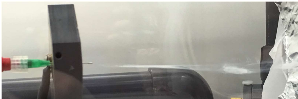
Figure 2.1. Self-bundling of PMIA nanofibers dissolved in DMAc/LiCl.
