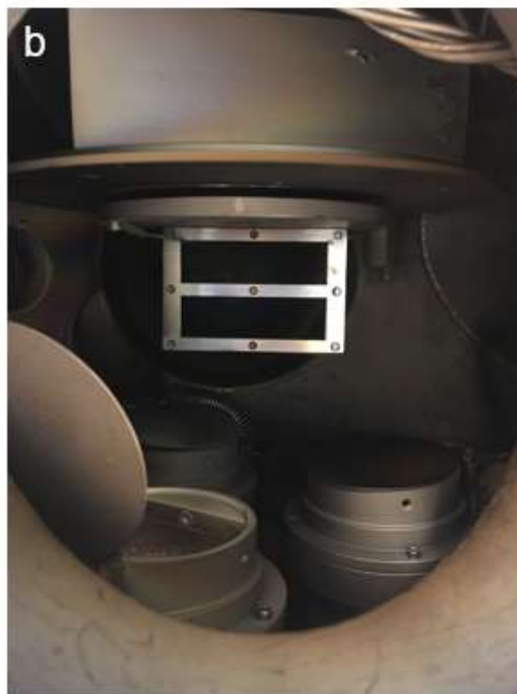
Figure 3.9. One step conformal sputter coating of copper experiment. (a) Scheme of one step conformal coating: Sample is rotating in front of the copper target. (b) Photo of the sputter coater with the sample loaded perpendicularly.
