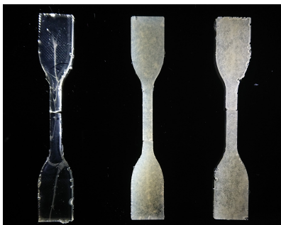
Figure 5.2.1: Representative Composite Dog Bones for Tensile Testing. From left to right: epoxy, Kevlar 49 reinforced composites, and PPTA nanofiber reinforced composites.
