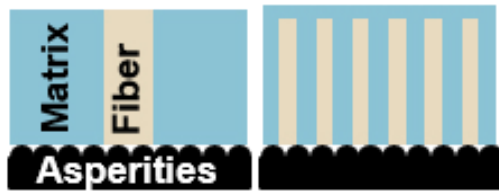
Figure 5.1.1: Length scale ratio of asperities to fibers will affect the wear rate by changing the mechanism of wear. When fibers are larger than the asperity, the asperity wear either the fiber or matrix one at a time leading to a volume wear rate. When fibers are the same size or smaller than the asperity, then the asperity will pull both the matrix and fiber at the same time leading to mechanical wear rate.
