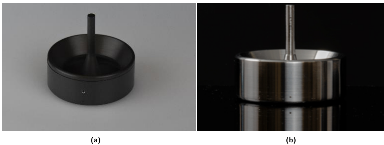
Figure 3.1.2: Continuous Loading Reservoirs for Engineering Continuous Fibers. a) Reservoir milled from Al 7075 and hard coated with anodized Teflon was engineered for spinning solutions with slight corrosivity at speeds up to 80k RPM and b) Hasetloy C276 reservoir was engineered to spin PPTA-sulfuric acid dopes up to speeds of 45k RPM.
