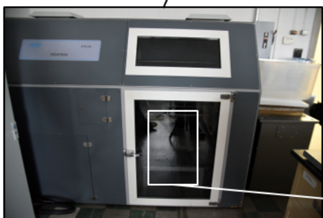
Figure 6.2.1: Abrasion Testing of PPTA Nanofiber Reinforced Polyurethane Boot Soles. a) A boot coated in PPTA nanofiber reinforced polyurethane as placed in an b) abrasion tester. To test the wear rate of the coated boot, the machine c) replicates the boot walking along a concrete bath. The concrete rotates to ensure the boot does not land in the same place every step 6.2.1.
