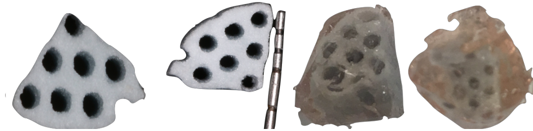
Figure 22. showing photos for the 3D printed porous calcium phosphate(CaP) block on the left, and the Gelatin-HPA Infused (CaP) 3D printed blocks.
