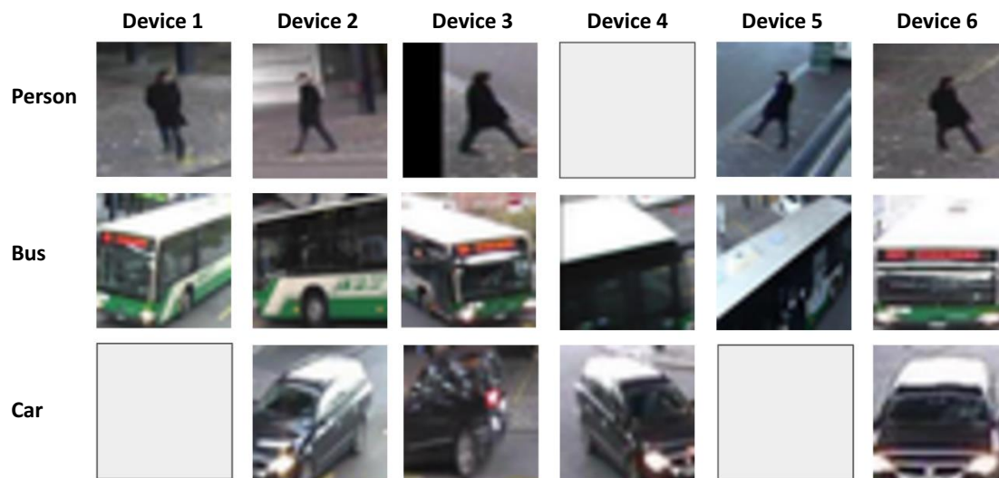
Figure 4.5: Example images of three objects (person, bus, car) from the multi-view multi-camera dataset. The six devices (each with their own camera) capture the same object from different orientations. An all grey image denotes that the object is not present in the frame.
