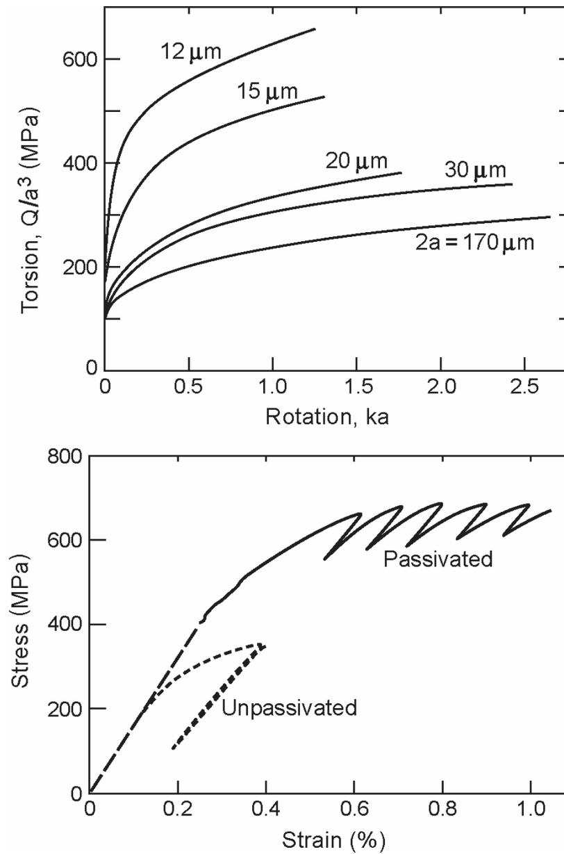
Fig. 3 Top plot: Normalized torque versus normalized rotation for copper wires of various radius,  $a$  [7]. This normalization would collapse the data to a single curve if there were no material size-dependence. Lower plot: Tensile stress-strain data for thin copper films ( $0.34\ \mu\text{m}$ ) that are unpassivated and passivated (on one surface) [9].
