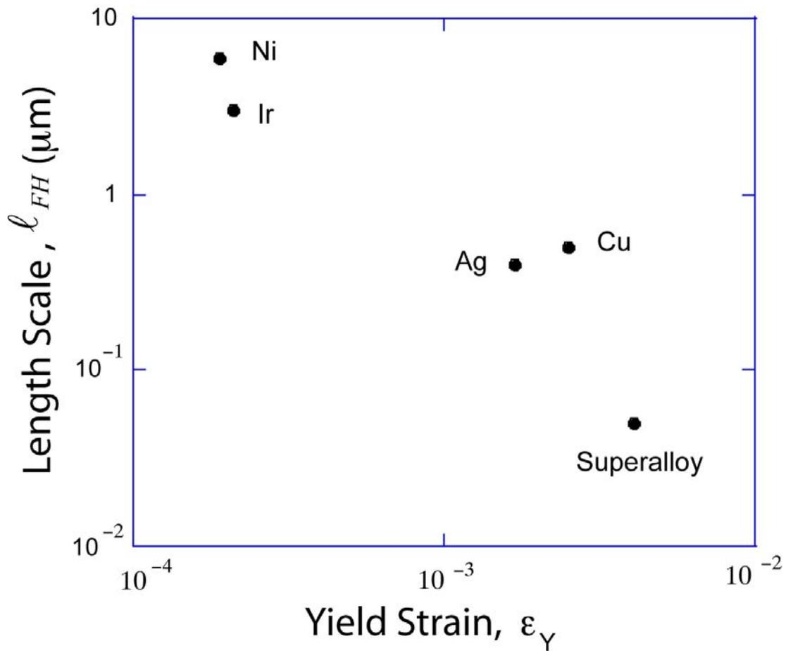
Fig. 13 A plot of the length scale,  $\ell_{FH}$ , against the size-independent tensile yield strain. The length scale was ascertained using FH theory using indentation data for Iridium [3], a superalloy [29], copper [5], and silver [2], together with the present finding for bending of Ni foils.
