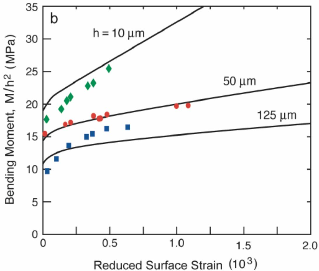
Fig. 12 Prediction from FH theory incorporating a strain-dependent length parameter,  $\ell(\varepsilon_p) = \ell_0(1 + a_0(\varepsilon_p / \varepsilon_Y))$ . The values,  $\ell_0 = 2 \mu\text{m}$  and  $a_0 = 0.2$ , were chosen to both fit the data for the foil with  $h = 50 \mu\text{m}$  at  $\varepsilon_r = 10^{-3}$  and to better represent the initial increase in strength and hardening of the foil with  $h = 10 \mu\text{m}$ .
