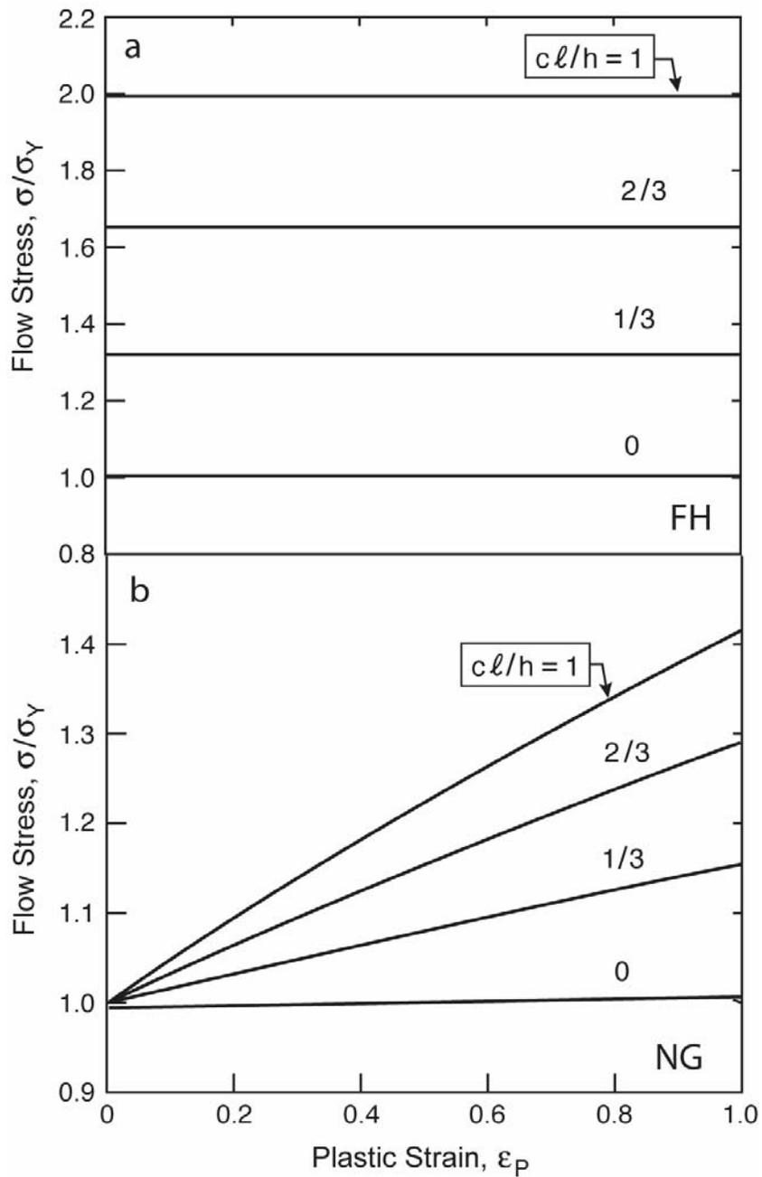
Fig. 4 Trends of average flow stress as a function of average plastic strain,  $\epsilon_p$ , for an object of size  $h$  subject to an average gradient of plastic strain  $\epsilon_p^* = c\epsilon_p / h$ . (a) FH and (b) NG formulations.
