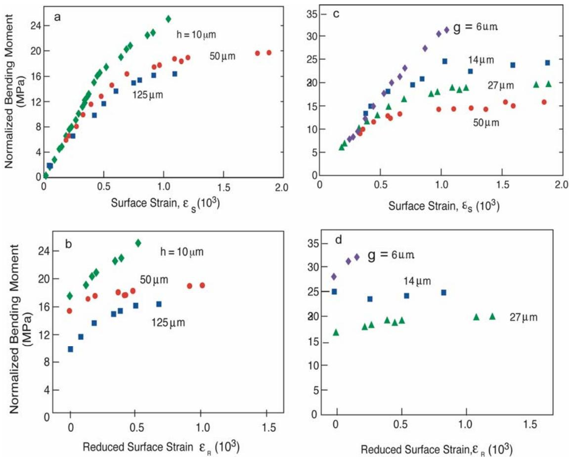
Fig. 1 Normalized moment,  $M/h^2$  as a function of surface strain,  $\epsilon_s$ , and reduced surface strain,  $\epsilon_r$ , for Ni foils. (a) and (b) For three thicknesses with grain size  $g = 27 \mu\text{m}$ . (c) and (d) For three grain sizes with foil thickness  $h = 50 \mu\text{m}$  [19].
