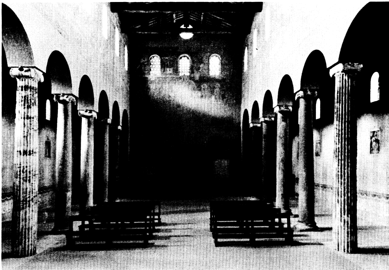
Figure 2. S. Giovanni a Porta Latina, Rome, 1191. The simple plan conforms to Roman basilicas of the fourth century. Columns, plinths, and some capitals are spolia.
