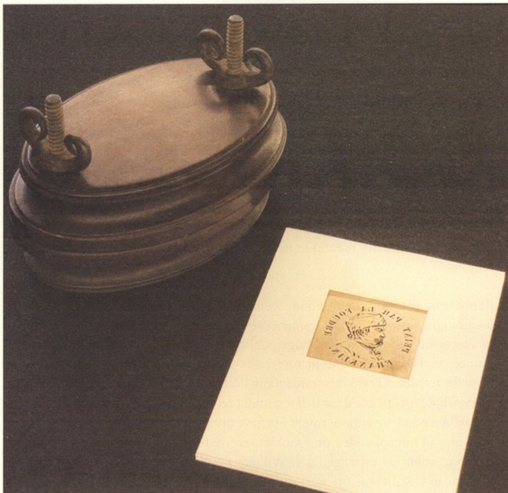
Figure 18. Electrical printing press and stencil, English, ca. 1760 (item 62). Reproduction courtesy of the Collection of Historical Scientific Instruments.
