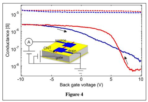
hole conduction<sup>13</sup>, while the metallic tube did not show a significant back gate hysteresis response. The commonly observed in ambient conditions for conventionally made SWCNT FETs<sup>14</sup> is noted.
