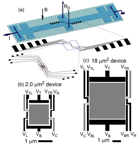
FIG. 1: Measurement setup and devices. (a) Diagram of the wet-etched Hall bar, surface gates, and measurement configuration. Diagonal resistance,  $R_D$ , is measured directly across the Hall bar, with current bias,  $I$ . Subsequent zoom-ins of the surface gates are also shown; the red box encloses the detailed gate layouts for the device shown in (c). (b,c) Gate layouts for the  $2.0 \mu\text{m}^2$  and  $18 \mu\text{m}^2$  devices, respectively. The areas quoted refer to those under  $V_C$ .
