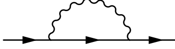
FIG. 6. Feynman diagram for the self-energy correction. The solid line with arrow represents F or G fermion propagator and the wiggly line represents electric field propagator. The interaction vertex is given by equation (3.12). This diagram is evaluated in equation (3.18).
