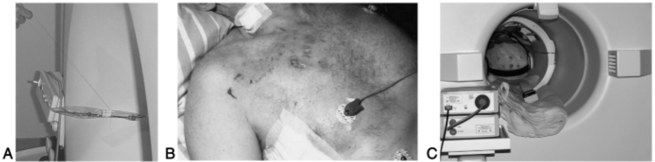
Fig. 3. (A) Magnetically-induced force attracting a metallic probe towards the magnet. According to standard safety criteria the deflection angle needs to be less than 45^\circ . Reproduced from Schaefer (2008) by permission of the copyright holder, IEEE. (B) Second-to-third degree burns on the thorax where ECG electrodes were applied, following an incident involving high-voltage induction in long leads. Reproduced from Kugel et al. (2003) by permission of the copyright holder, Springer-Verlag. (C) Reducing lead length, running the conductive wires in parallel near the centre of the magnet and using appropriate padding minimizes risks and improves signal quality. Reproduced from Herrmann and Debener (2008) by permission of the copyright holder, Elsevier.
