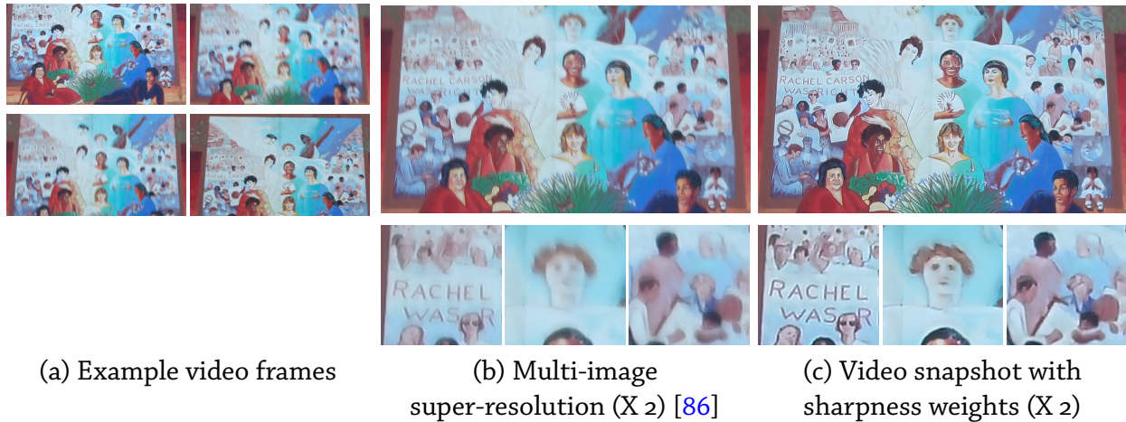
Figure 4.5.2: Video snapshots for motion blur. Often when photographing a scene with a moving camera, some of the frames, possibly even the desired frames captured, are motion blurred. (a) This is illustrated on this video clip of a mural captured with a hand-held video camera (21 frames, 640 \times 360 resolution), where the reference frame has the best composition of the scene, but is motion blurred. (b) Most of the frames in this video clip are blurred and combining all of them to super-resolve the reference frame [86] results in a blurry image. (c) Using the local sharpness weights in our framework ensures that pixels from only the sharp frames are propagated to the reference frame, resulting in a sharp snapshot.
