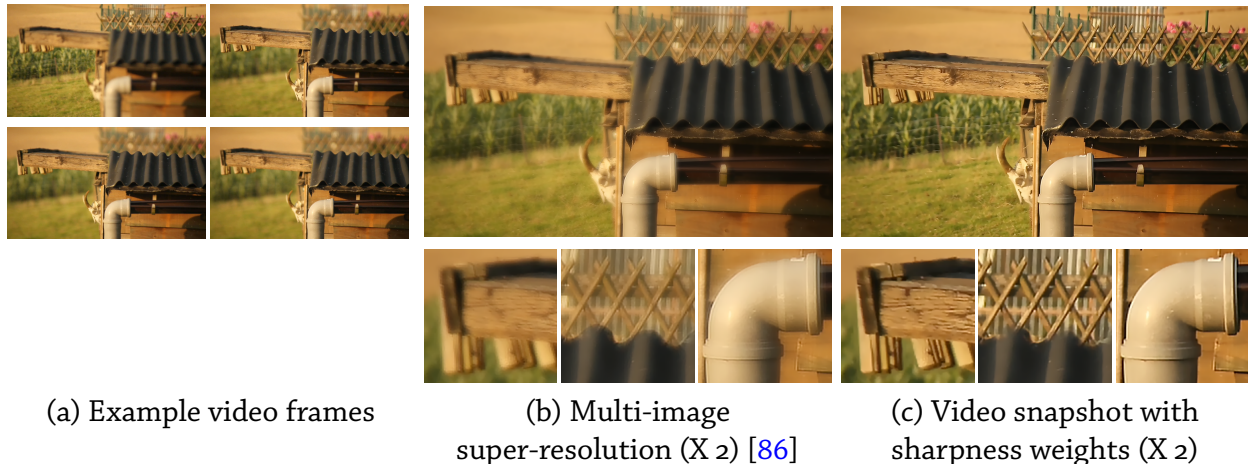
Figure 4.5.3: Video snapshots for defocus blur. (a) In this video clip (21 frames, 640 \times 360 resolution), shot with a handheld video camera, the focal plane is being moved from the back to the front to create an unstabilized focal stack. (b) Naive multi-image super-resolution [86] combines both sharp and blurry frames, and produces a result that is only marginally sharper because it does not model the defocus blur in the video properly. (c) Our result uses local sharpness weights to identify and combine the sharpest pixels in the input video clip to produce an all-in-focus super-resolved snapshot.
