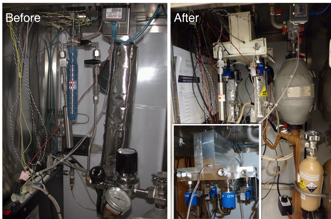
Figure A.14: Cambridge Nanotech Savannah 100 ALD system before and after converting it from two Parker valves (aluminum precursor on one, \text{H}_2\text{O} and \text{NO}_2 on the other) to four Swagelok valves ( \text{H}_2\text{O} , aluminum precursor, hafnium or zirconium precursor, and \text{NO}_2 or IPA) with improved heating of precursor lines. Inset: valve assembly and heater block before application of thermal insulation and attachment of precursor cylinders.
