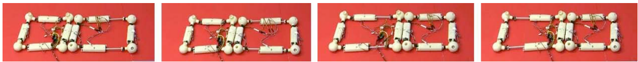
FIGURE 7: 2-SQUARE ROBOT IN MOTION: THROUGH LINEAR ACTUATION THE ROBOT IS ABLE TO SHIFT ITS WEIGHT AND CRAWL FORWARD.
