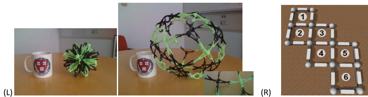
FIGURE 9: OTHER POTENTIAL EXPANDABLE STRUCTURES: (L) HOBERMAN™ SPHERE, WHERE THE SCISSOR-LIKE LINKS BEHAVE SIMILAR TO AN ACTIVE LINK THAT CHANGES LENGTH. (2) AMORPHOUS 2D ROBOT COMPOSED OF SQUARE UNITS [6].
