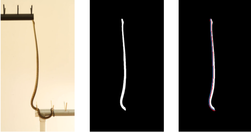
Figure 4.2: A sample of how the image analysis process works. We take an image from the video (left), crop it and edit out the top and bottom perches. Starting from the cropped image (center) we use our image analysis software to extract the front of the body (right). In red are points representing the pixel values of points on the front of the snake. The blue line is an interpolation through the pixel values. We use the interpolated line to compute curvature because the raw pixel data is too noisy.
