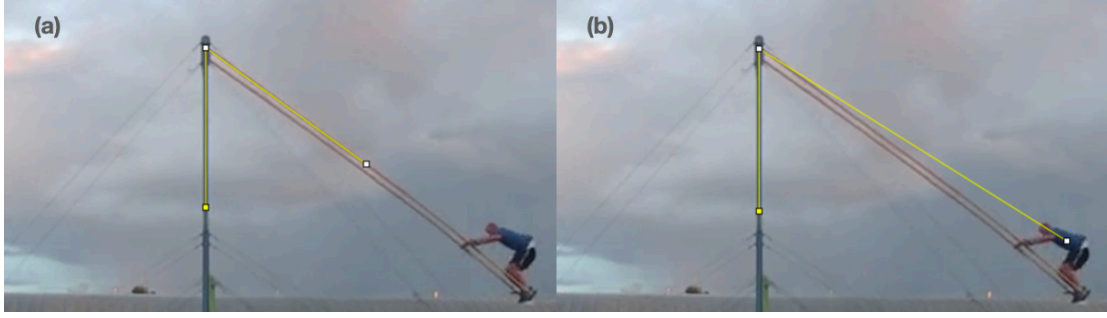
Figure A.1: Measuring angles with image analysis software Fiji 85 . We approximate the mass of the swing structure and the athlete to create a weighted average of the system center of mass. The angular location of the true center of mass is somewhere in between the post the athlete is holding and the athletes torso. The difference in measured angles provides an upper bound on the measurement error. (a) Measuring the angle the swing makes with the vertical. (b) Measuring the angle between the approximate center of mass of the athlete and the vertical.
