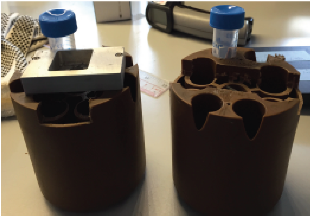
Figure 3.8: Modified centrifuge buckets for holding sample cells during centrifugation.
