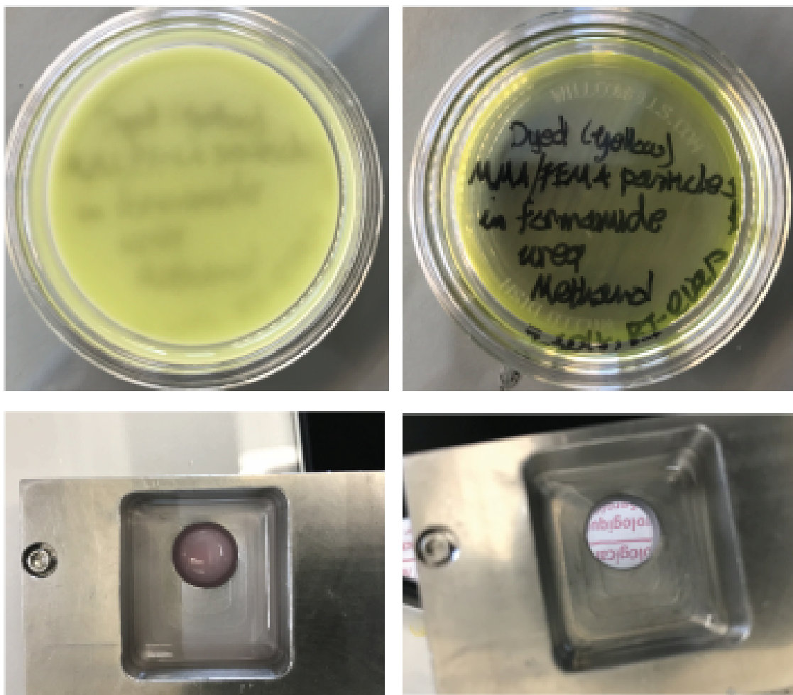
Figure 3.7: Evaporation of methanol from methanol-formamide solution to restore refractive index matching
