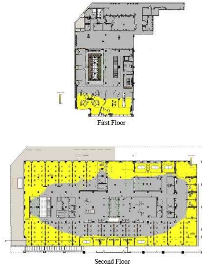
Figure 15. Daylight autonomy analysis of model office space.
