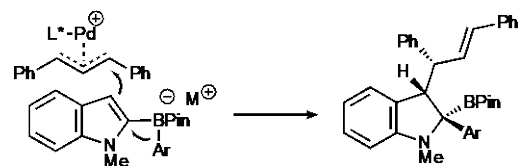
Figure 2.5 Catalytic, enantioselective rearrangement of vinyl boronates
