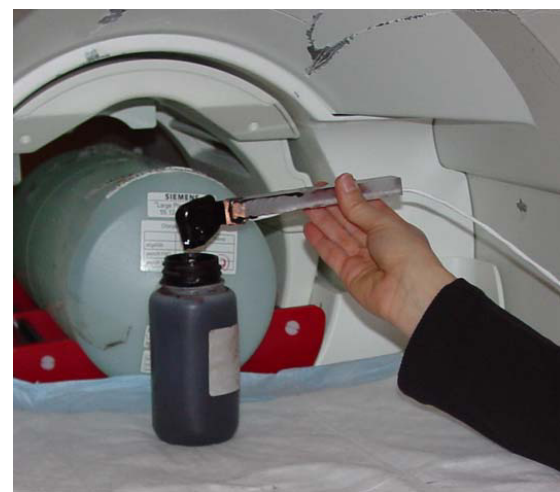
Figure 6 Simple device that was used to test the MR compatibility of ERFs.
