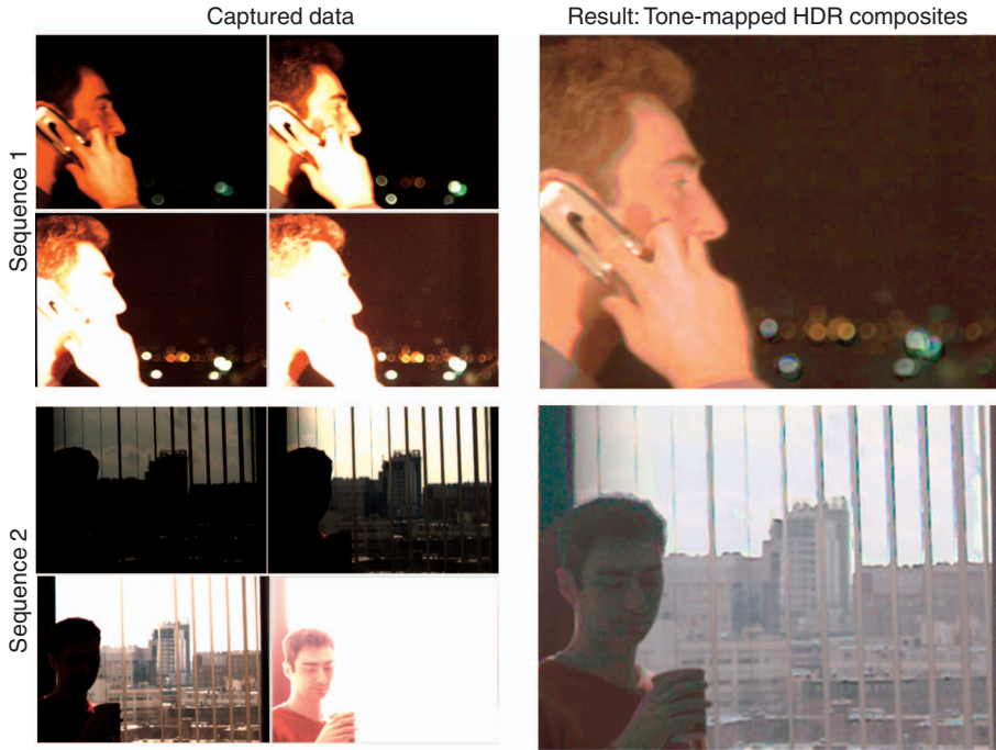
9 Frames from two HDR sequences. Images on the left are four simultaneously captured views. The large images on the right are the corresponding tone-mapped composites.
