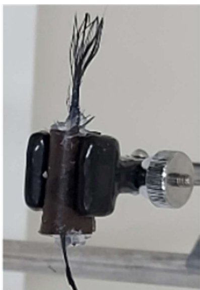
Figure 3.11: Flexible battery performance of 2-BEAQ. a. Photograph of a wearable gel battery containing 2-BEAQ negolyte and ferrocyanide in xantham gum posolyte at pH 14. b.
