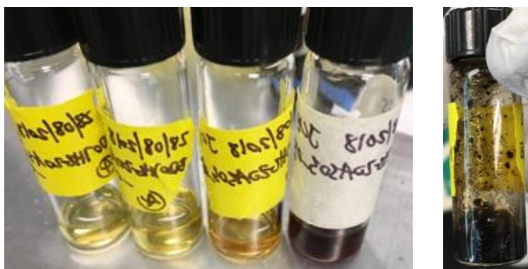
Figure S1-17. Series of 0.4 M BD/0.2 M AS solutions at increasing time of reaction rightward (left). 0.4 M BD/0.2 M AS solution after weeks of reaction (right). Solutions had approximately the same starting composition. The solutions darken over time and solids appear to form. A visible color change to a darker yellow was observed within minutes. Black-brown color was noticeable after hours of reaction. The accumulation of solids occurred on longer timescales (many hours to days). Solids were also observed rapidly (under an hour) in BD/NH x solutions with higher pH (e.g., in BD_NH_pH8.5 experiments).
